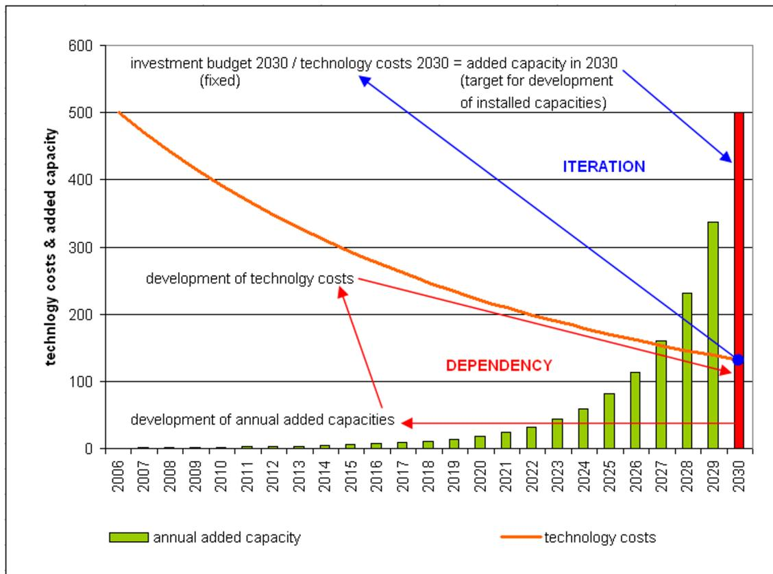
Figure 6: Example of translating the 2030 investment budget into new added capacities in 2030 with regard to degression of specific technology costs (see also Figure 5 on page 17 for more information on iterative technology cost calculation). [S. Peter, H. Lehmann; 2007]
